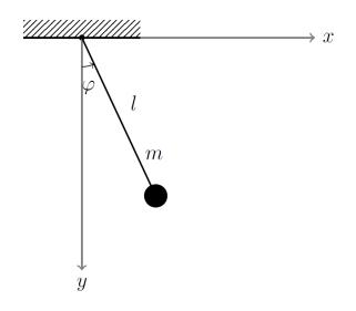
Analysis of the scheme allows to claim its number of degrees of freedom which is 1
